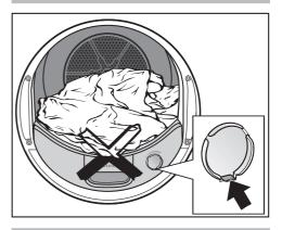
If you are not using a fragrance flacon: the tab must be pushed down completely (see arrow).
